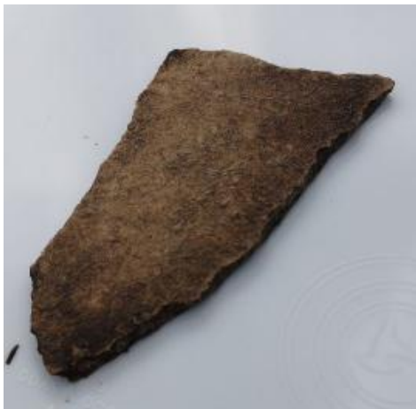
Faserzementplatte, grau (Probe 2):
